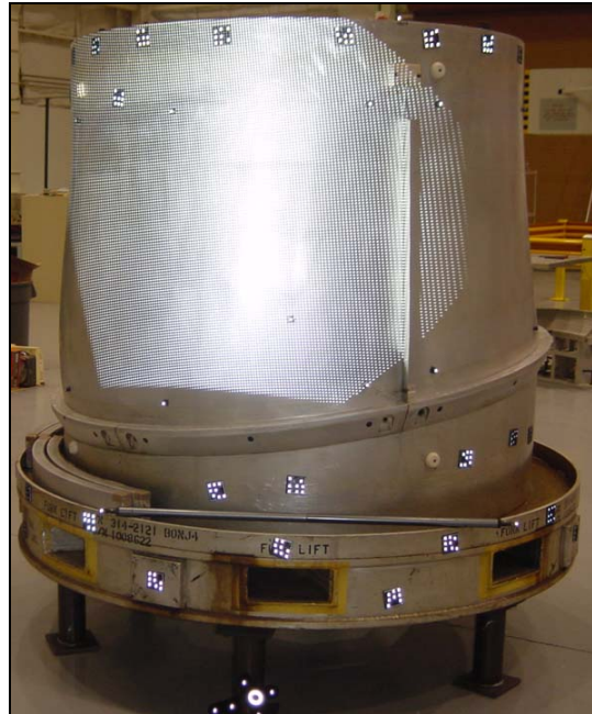
737-700 Lay up Tool Measured.
