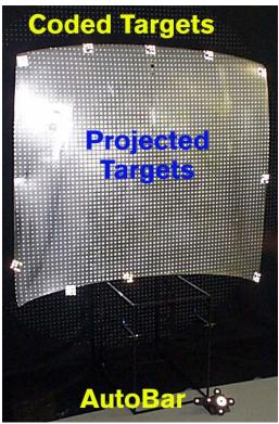
single-camera is used to take pictures from two or more different locations around the object. Each time a picture is taken, the stroboscopic projector also projects the pattern of high-contrast dots onto the surface.
